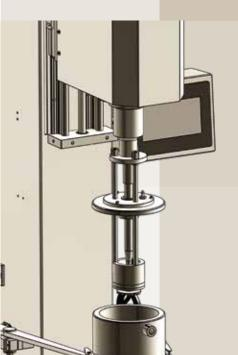
**VBR Series Dispersers** are actually **Multi-Purpose** machinery, designed for all kinds of pre-mixing, ready mixing, dispersion / dissolving, homogenizing and milling processes for laboratory scale, within a wide viscosity range of products. The machine can be used as a laboratory scale **Dissolver, Basket Mill** and **Roto-Stator High Shear Mixer** with its interchangeable workheads.
